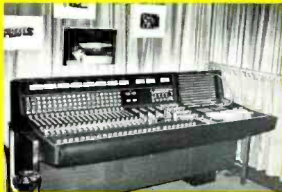
Automated Processes has a large patch bay in their 20-in, 16-out console. Circle 51 on Reader Service Card.
