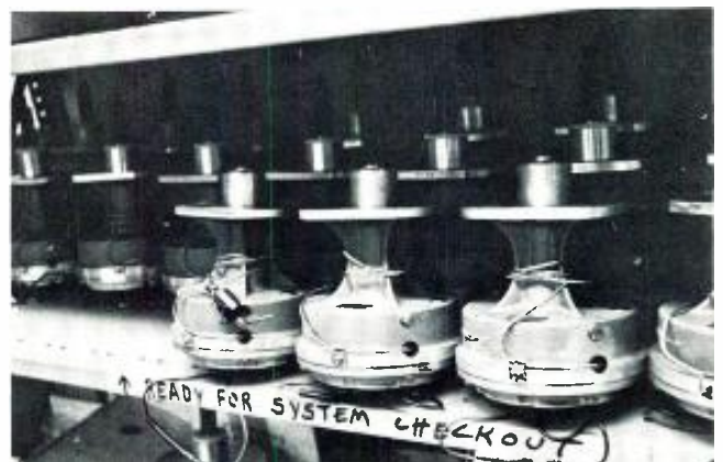
Special d.c. capstan motors used in the ABR stand ready for inspection.
